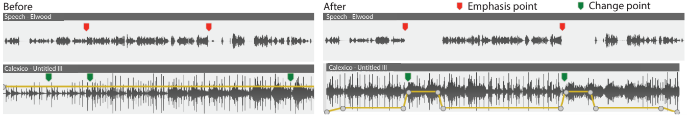
Figure 6. In constrained music retargeting, the producer selects multiple speech emphasis points (red markers) and a piece of music (before). Our system automatically identifies music change points (green markers) and aligns them with the emphasis points, by extending or shrinking the music as necessary, while preserving the local beat-level structure of the music (after).
