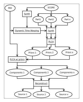
Figure 1. Architecture of the score-informed PLCA-based source separation system
